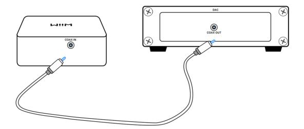
Note: The COAX In interface on the WiiM Vibelink Amp supports PCM audio format only. Please ensure that the audio source device connected to the WiiM Vibelink Amp is set to output audio in **PCM** format. Otherwise, you may not hear sound.
